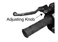
The adjustment range is limited. Never apply excessive force to the knob. Always turn the knob manually.
